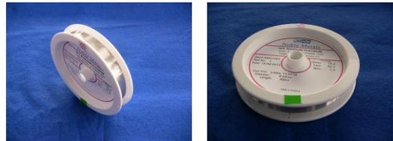
3. The wire should be stored on the reels it was supplied on and any supporting bands remain on the wire until it is used, and replaced if needed.
