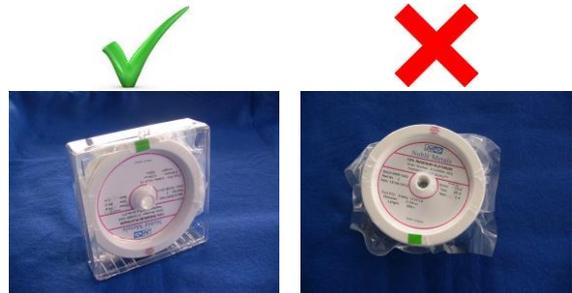
2. The reels should be stored in the 'rolling position' to ensure that the layers of wire do not tangle.
